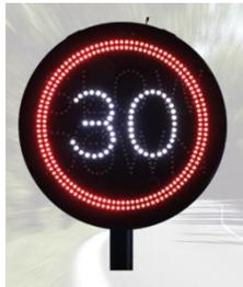
230V LED Vehicle Activated Sign displaying, when activated by an integral MVD, (Microwave Vehicle Detector) diagram 670 (XXMPH client to confirm) in Red & White LED's. The sign will alternate between this and a warning message reding SLOW DOWN in white LED's. The sign body is to be of black powder coated aluminium construction with channel to rear to allow for post mounting. (Client to confirm post diameter)
