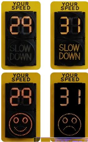
230V mains or 12V powered (Depending option ordered), Mini 300 SPEED DISPLAY, polyurethane bodied modular sign c/w a Yellow Non-Reflective border and "YOUR SPEED" text The Inter-active sign will display a 200mm real-time illustration of the approaching speed of an oncoming vehicle. When exceeding a pre-set threshold limit, the sign will display a "SLOW DOWN" safety message in Amber LED's. Or a Sad/Smiley face depending on the option you choose.
